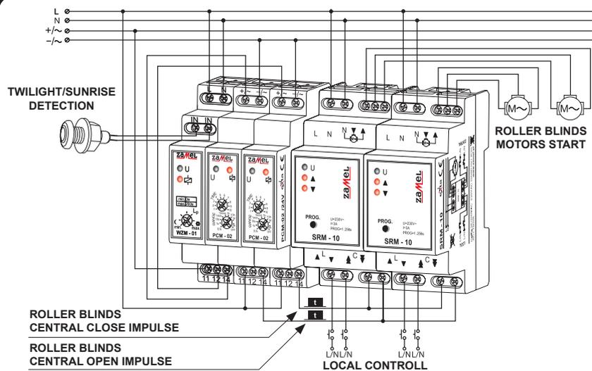
The relay PCM-02/24V cooperating with a twilight switch WZM-01 and roller blinds controllers SRM-10 must generate an impulse after detecting twilight. The impulse is a signal for the roller blinds controller (central closing input) to shut all roller blinds operating in one group.
