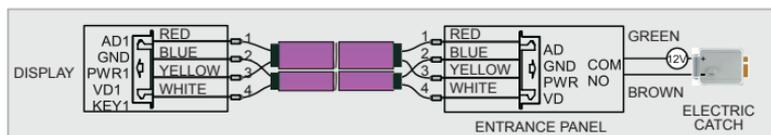
If the open command is output by a display, use this wiring specification:
