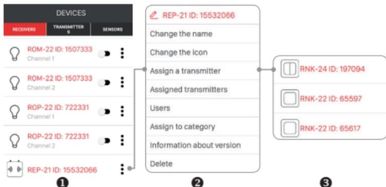
Remote assigning of transmitter to the repeater can be also executed from the transmitter level. In this case, select "Assign Receiver" option from edit menu of the transmitter.
