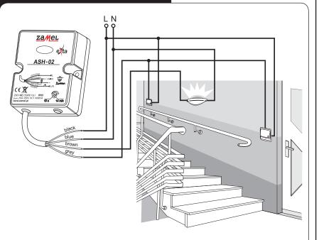
The staircase timer controls the staircase lighting and operates in four-conductor wiring configuration. It is possible to connect the single pole push buttons (e.g. illuminated) in parallel.
