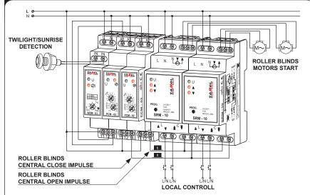
PCM-02 time relay cooperates with the WZM-01 twilight switch and with SRM-10 roller blinds controller. Its function is impulse generation at dusk. This impulse is a signal for the roller blinds controllers (central closing input) and for moving down all the roller blinds working in the same group.
