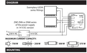
CAUTION! The device is designed for single-phase installation and must be installed in accordance with standards valid in a particular country. Installation, connection and control should be carried out by a qualified electrician staff, who act in accordance with the service manual and the device functions.
