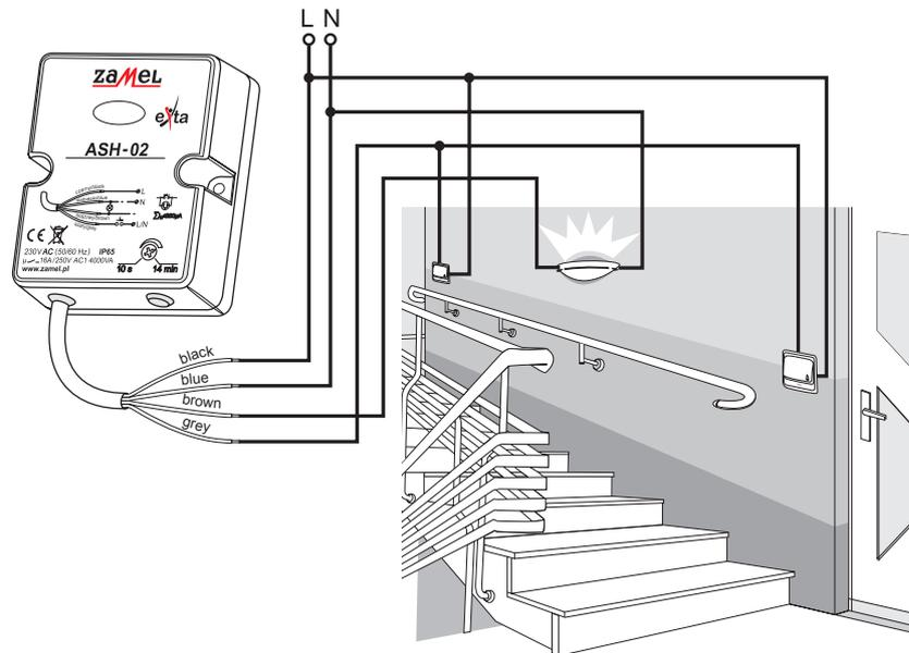
The staircase timer controls the staircase lighting and operates in four-conductor wiring configuration. It is possible to connect the single pole push buttons (e.g. illuminated) in parallel.
