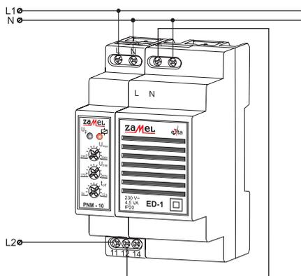
Control and L1 phase voltage drop signalling circuit.
