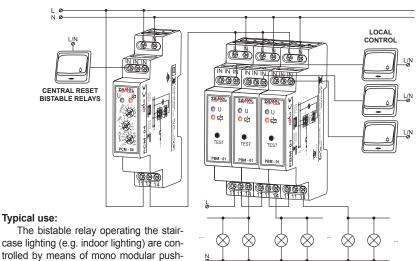
The bistable relay operating the staircase lighting (e.g. indoor lighting) are controlled by means of mono modular pushbuttons that can be connected in a parallel
