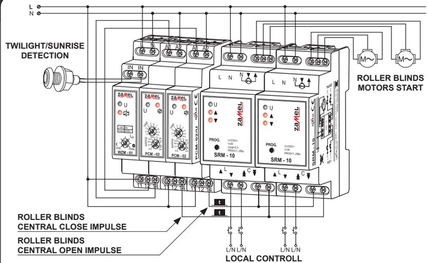
PCM-02/U time relay cooperates with the ZWZM-01 twilight switch and with SRM-10 roller blinds controller. Its function is impulse generation at dusk. This impulse is a signal for the roller blinds controllers (central closing input) and for moving down all the roller blinds working in the same group.
