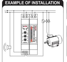
PNM-10 voltage relay cooperates with the LDM-10 voltage indicator. The value of voltage in a single-phase network is measured in the circuit of the relay whose outputs cut off the power supply to the protected circuit (e.g. motor) if the set voltage range has been exceeded. Voltage indicator allows ongoing visualisation of value of voltage supplying the protected circuit.
